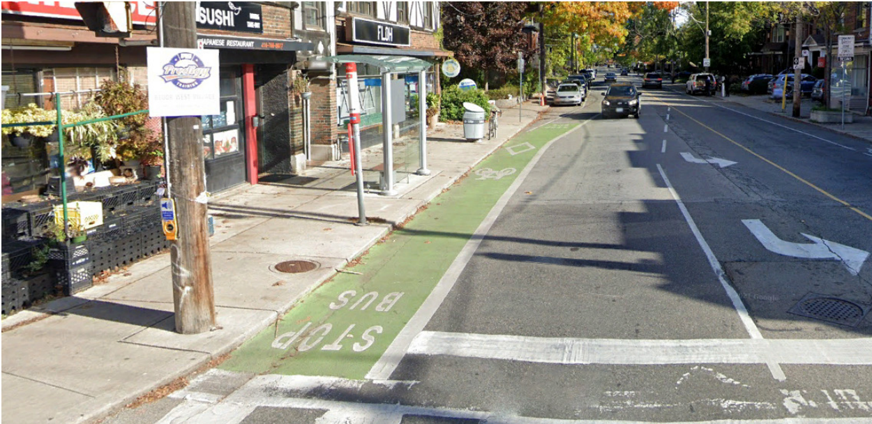
Shared space bus stop in Toronto. Source: Google Earth
