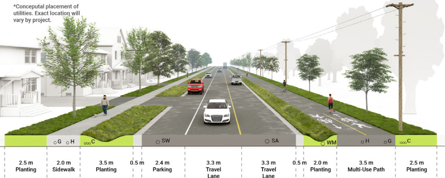
Typical Rural Settlement Area Cross Section with a Multi-Use Path (26m ROW)
