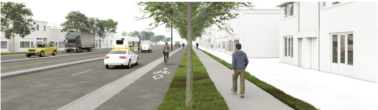
Planting zone between cycle track and sidewalk
