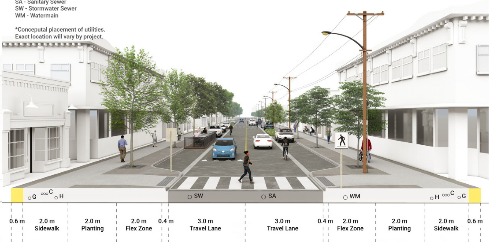
Typical Main Street Cross Section (20m ROW).
